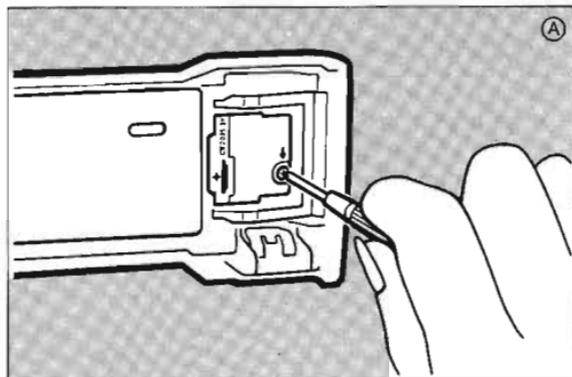
When the "BATTERY" mark lights up in the display panel, the battery has become exhausted. Replace promptly as directed.
